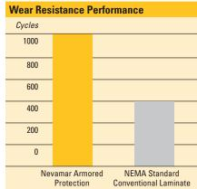
Armored Protection gives Nevamar laminates more than twice the wear protection than standard laminates. (ANSI/NEMA LD3 test method)
